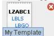
Press the icon of a saved template and the template data will be filled in the fields of the currently edited flight plan. The time fields shall not be completed. A template can be deleted by pressing the red button
